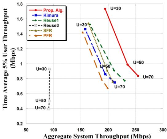
Figure 2. Edge TATP Vs ATP for (30,50,70) users/cell with 3Mbps/user.
