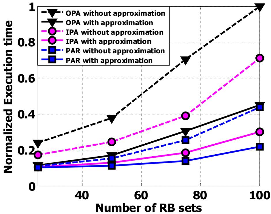
Figure 7: Normalized Execution time for OPA, PAR, and IPA with/without Hessian approximation
