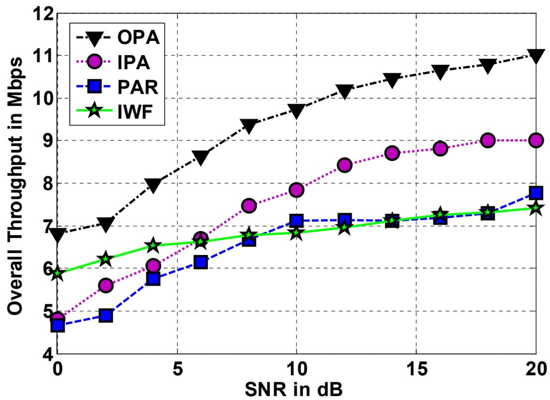
Figure 2: Overall throughput for OPA, PAR, IPA, and IWF assuming CS
