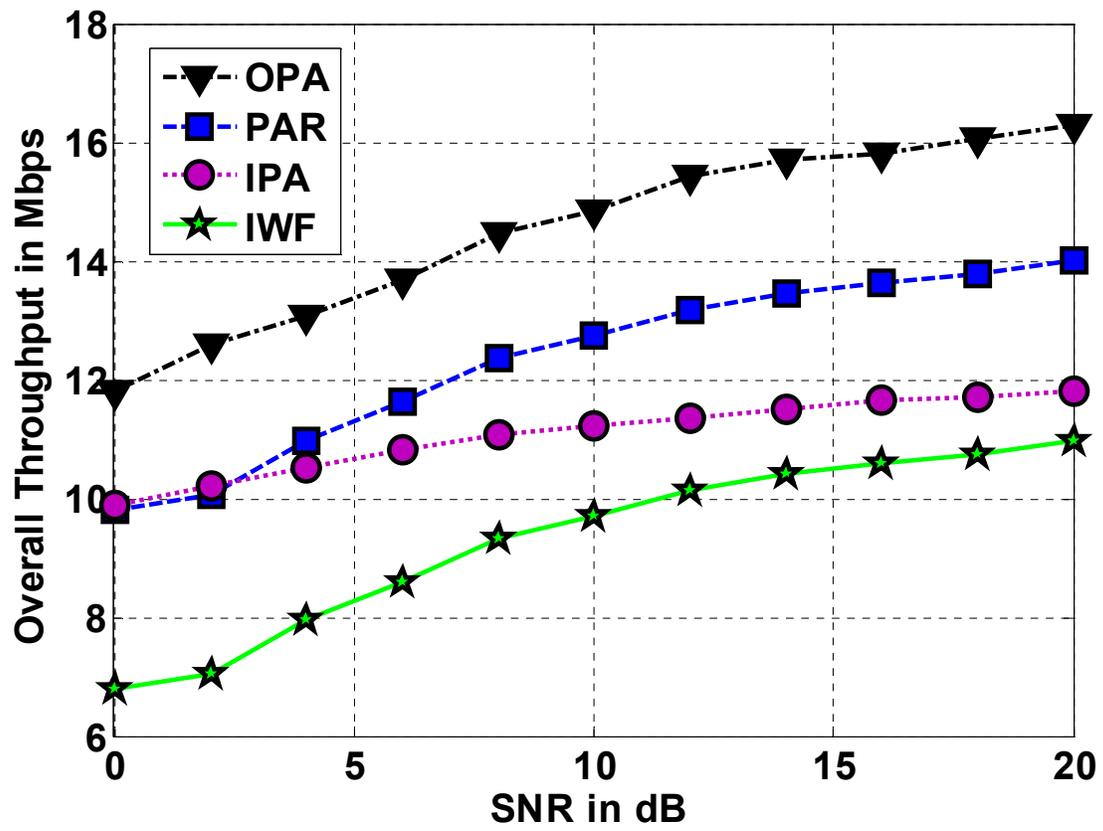
Figure 3: Overall throughput for OPA, PAR, IPA, and IWF assuming JP.
