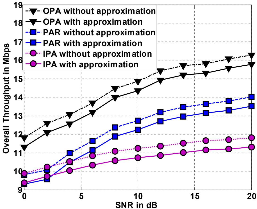
Figure 9: Throughput for OPA, PAR, and IPA with/without Hessian approximation assuming JP.
