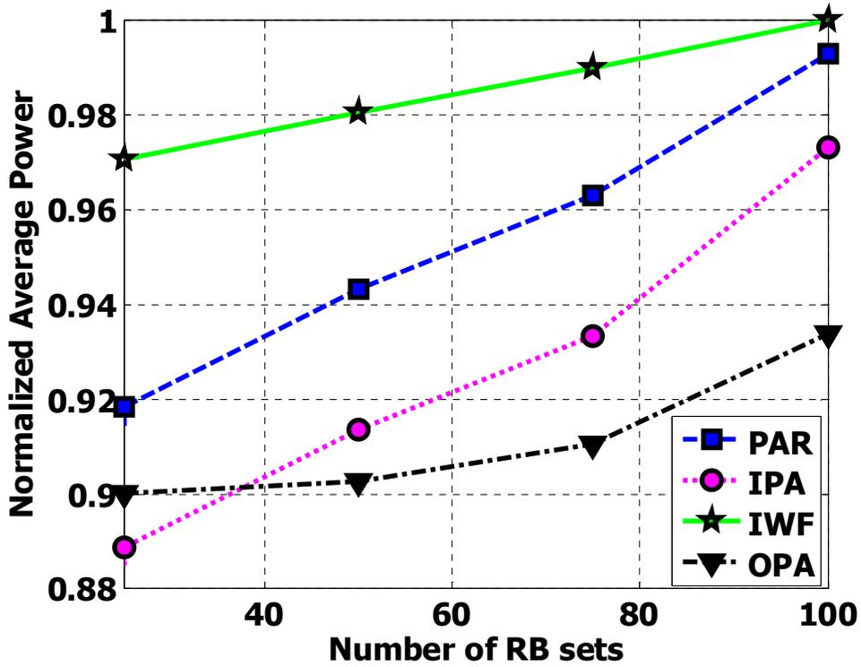
Figure 4: Normalized average power for OPA, PAR, and IPA.
