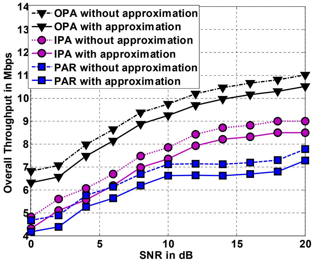
Figure 8: Throughput for OPA, PAR, and IPA with/without Hessian approximation assuming CS.
