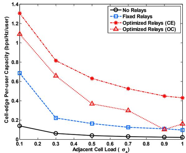
Figure 13: Cell-edge Per-user capacity vs. Adjacent Cell Load.
