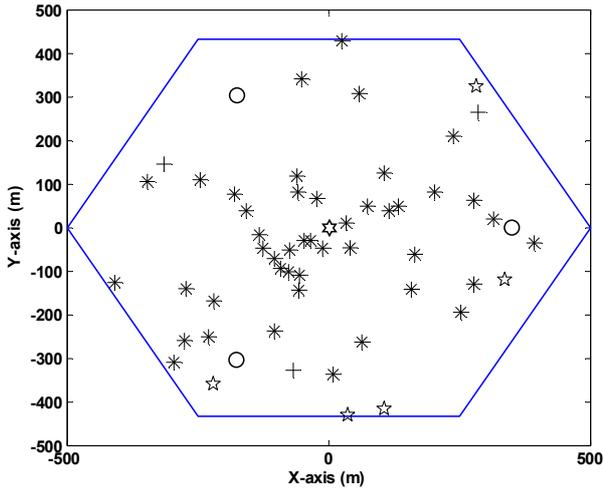
Figure 10: Optimal RS placement for the total cell capacity objective function.
