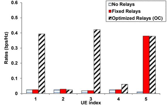
Figure 8: Rates of cell-edge users at  $\sigma = \sigma_A = 1$ .
