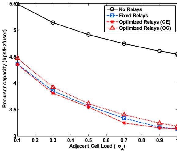
Figure 14: Per-user Capacity vs. Adjacent Cell Load.
