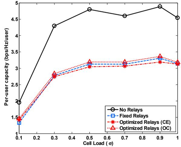
Figure 12: Per-user Capacity vs. Cell Load.
