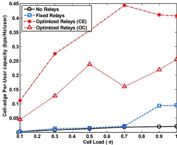
Figure 11: The Cell-edge Per-User Capacity vs. Cell Load.
