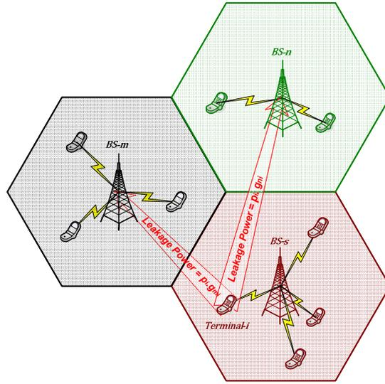
Figure 1: System model illustrating the concept of leakage power to neighboring cells
