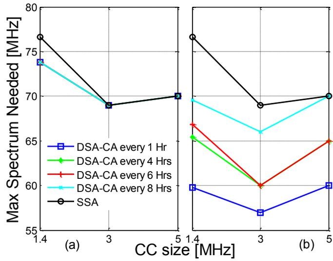
Fig. 6. Maximum Spectrum Needed in case of (a) scenario 1 and (b) scenario 2.
