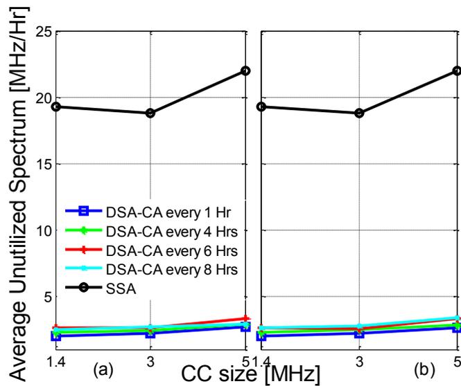
Fig 5. Average unutilized spectrum in case of (a) scenario 1 and (b) scenario 2.
