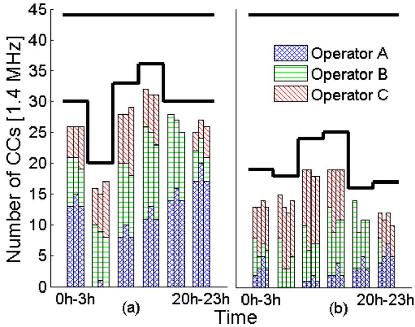
Fig. 4. The CCs required from different cells for Scenario 2 in (a) R1 and (b) R2. The black stairs show the actual CCs required to cover the demand from all cells over four-hour periods. The straight black line shows the CCs required in case of SSA
