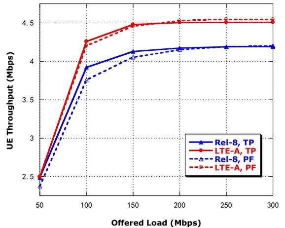
Figure 6. Average Rel-8 UE throughput and average LTE-A UE throughput (50% of users are LTE-A, rest are Rel-8)
