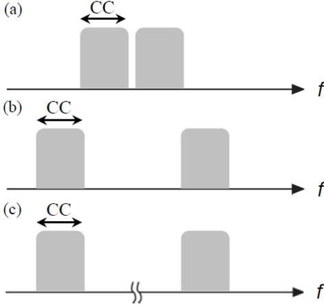
Figure 1. Carrier aggregation spectrum configurations: a) intra-band contiguous; b) intra-band non-contiguous; c) inter-band non-contiguous.
