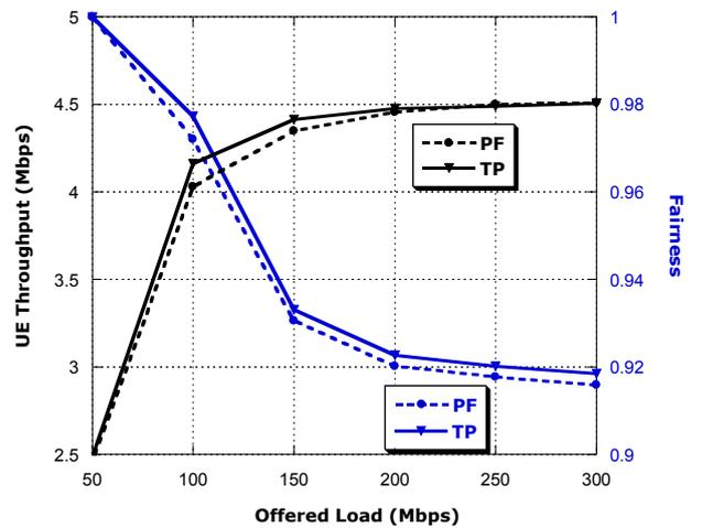
Figure 5. Average UE throughput and Fairness (50% of users are LTE-A, rest are Rel-8)
