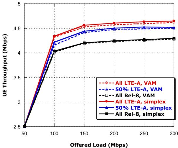
Figure 7. VAM versus simplex method in obtaining average UE throughput
