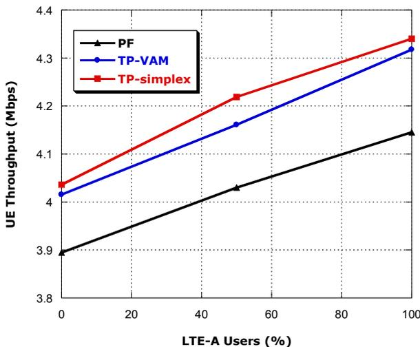
Figure 8. Average UE throughput versus percentage of LTE-A users for different schedulers
