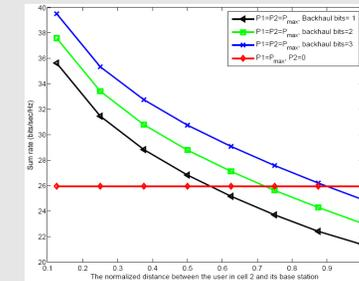
Fig. 2 This figure shows the sum-rate versus normalized distance for several numbers of quantization bits for the unequal distance case
