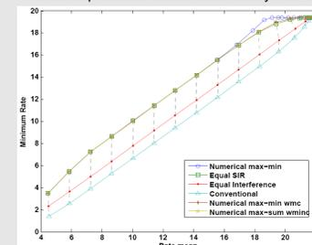
Fig. 3 This figure illustrates the minimum rate versus mean rate for several fairness schemes.
