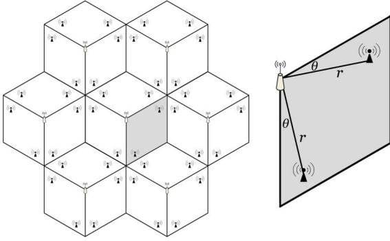
Fig. 2: RNs Deployment in a Cellular Network: (a) 7-Cell Layout and (b) RN Deployment per Sector
