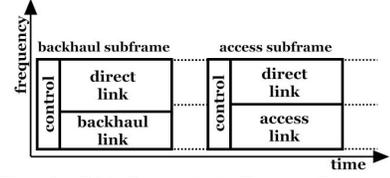
Fig. 3: RN Downlink Frame Structure
